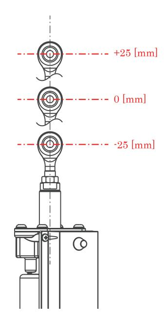
Fig 2.5 Definition of servo stroke positions
