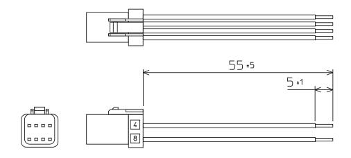
Fig 5.2 LJ9DA41 Cable (unit : mm)
